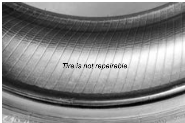
Example Internal Indication of Run-Low/Flat: Wrinkling of Innerliner in Shoulder Area
