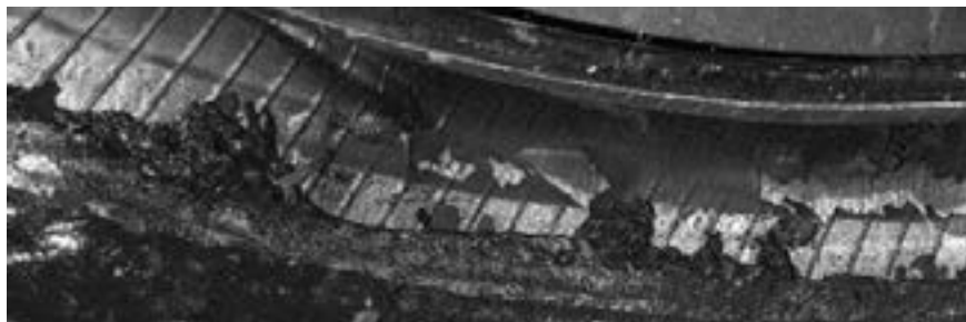
Tire is not repairable.
