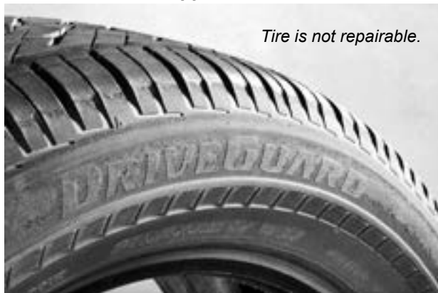
Example External Indication of Run-Low/Flat: Abrasion of Mid/Upper Sidewall and Shoulder
